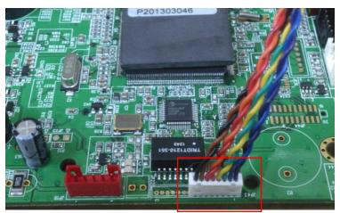
Note: This internal Ethernet interface only supports with the main board that has print server function on board.
