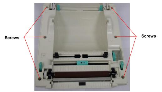
Remove 6 screws from lower inner cover
