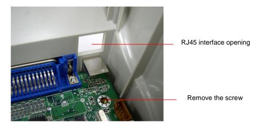
2. Remove the screw from the main board. Fasten the copper pillar and plastic pillar.
