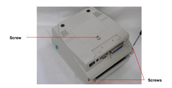
3. Remove 6 screws on lower inner cover.
