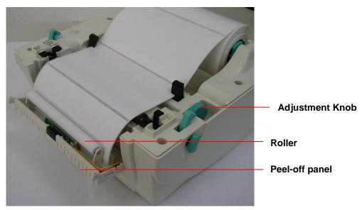
Loading label for peel-off mode
