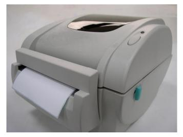
Label installation in cutter mode completed
