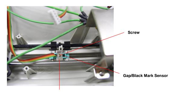
Gap / black mark sensor fixing plate
